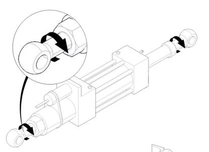
Check the distance between the welded beam attachment centres. If it is necessary, adjust the length using the rods.
