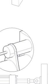
We recommend that you put the hydraulic shock arrestor with the oil reservoir in the upper side.
