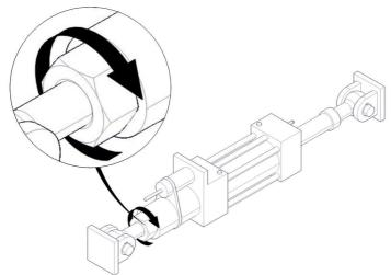
Finally, screw tightly the check nut.
