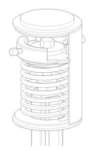
If the pins are leaning upwards (used to come like that after manufacturing), it means that the spring is pushing upwards stronger than the pipe downwards, and the spring must be tightened.
