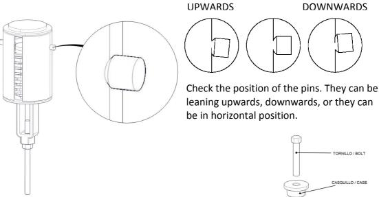
The turnbuckle is welded to the bolt. The bolt rests on the case, and the case over the plate.
