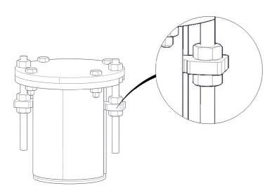
Once all the accessories are assembled (clamp, forged eye nut, rods, forged clevis, lug...), you must move the lower nut downwards (after the hydraulic test is finished).
