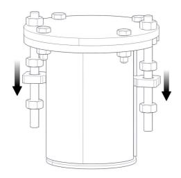
Tighten the spring using the turnbuckle (supports type A, B, C, E), the spindle (supports type F), or the regulator nut (supports type D) until the plate 2E moves slightly downwards. Then, screw the upper nut upwards.
