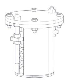
The blocking mechanism of these springs does not depend on the spring type. Anyway, it can be enlightening to read the corresponding assembly and unlocking guide for variable spring supports.
