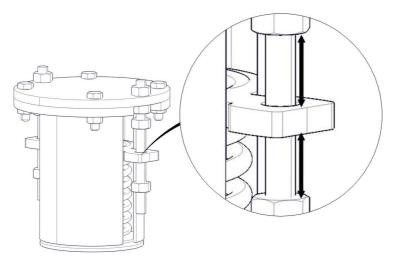
You should have into account that the plate will move from the installation position to the working position. This movement can be upwards or downwards. So you must move the upper nut upwards, and the lower nut downwards having into account the displacement.
